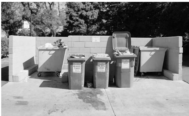
FIGURE 3.4 Typical example of containers used for low- and medium-rise apartments. Large containers are used for solid waste to be disposed of in a landfill. The smaller containers in front of the enclosure are used for: (1) glass, tin can, aluminum cans, and plastic containers (type 1 and 2) and (2) recyclable paper and paperboard products.
